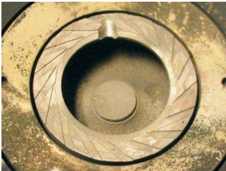
Figure 4: The heat insulated combustion chamber
