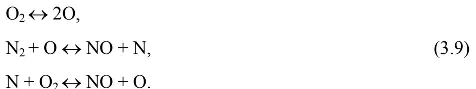
The last reaction is determinative and its rate depends on concentration of elemental oxygen. Calculation of NO formation is performed by chain mechanism for a combustion zone, then average NO concentration on whole cylinder volume
