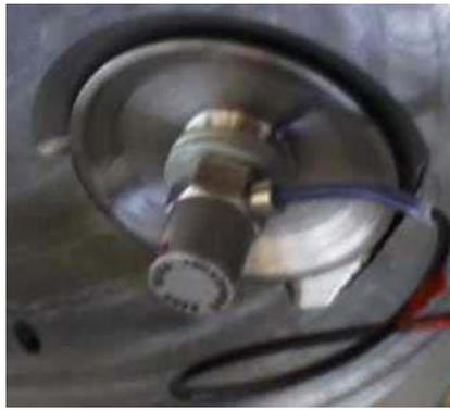
Fig. 4.4. The accelerometer mounted on the inlet valve
