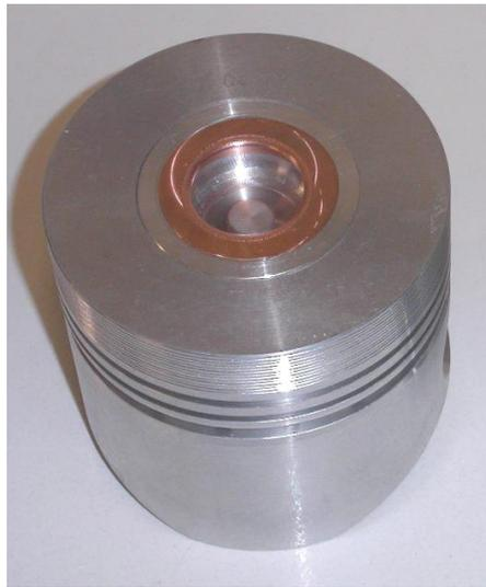
Fig. 4.8. Piston of the *Z-engine* prototype
