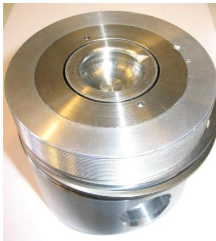
Fig. 4.11. The piston with the heat-insulated CC of the *Z-engine*
