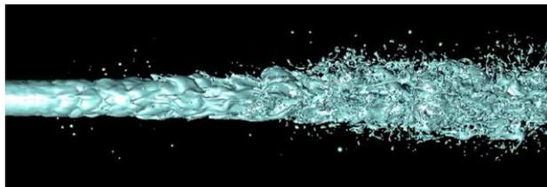
Fig. 2.63. The visualization of jet primary break-up obtained at *CFD* simulation in work [155]
