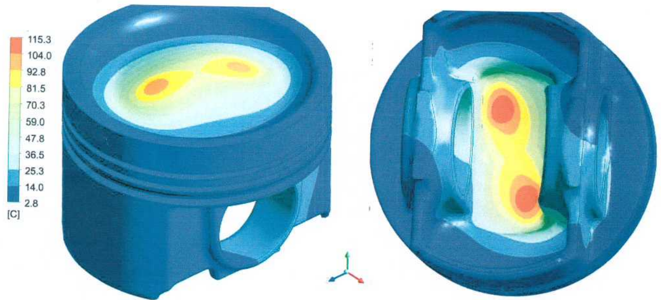
Figure - 67 Temperature difference due to type of cooling system - combined and with cooling channels
